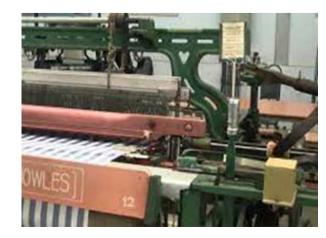
counter that can be used in shuttle based power looms. If a warp threads breaks or overlaps another or the weft pirn is about to exhaust itself of thread this device will stop the machine through electromagnetic actuated brake, with a display of the type of fault and sound an alarm.
